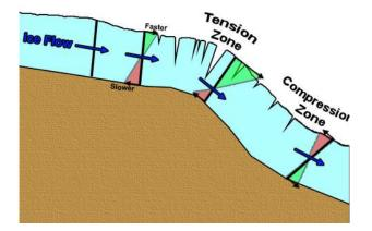
Figure 1: Ice moving over uneven bed.
