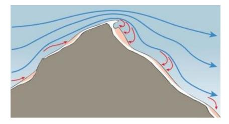
Figure 3: Flow lines of wind over a cliff and the formation of a cornice. Red arrows show slower windspeed.
